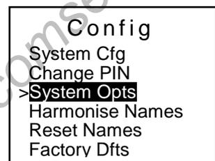
4. The 'System Opts' menu is displayed and the 'Latch Faults' option is highlighted.
