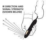
DO NOT COVER THE MAIN TRANSMITTING AREA WHEN PRESSING THE BUTTON (SHOWN ABOVE)
