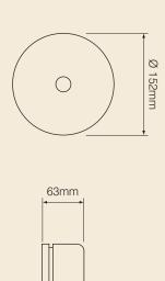
Bells still remain a popular choice for many applications such as schools where they can sometimes be used as a signal for non fire purposes such as class change. All CF bells incorporate highly efficient rotary centrifugal movements combining high sound output with low current consumption.
