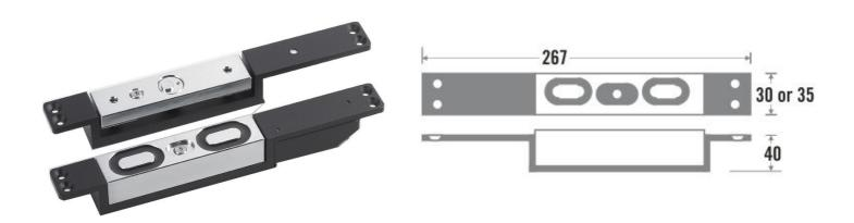
SL705-30 / 35 provide up to 2700lbs of shearing force. Suitable for metal or wood doors. Combines the best in failsafe performance with the most advanced features in shear lock design. With built in field adjustable automatic relock switch with a 1 to 6 second relock time delay. Working on 12V to 28VDC in put which is self selecting. PLEASE NOTE: Holding force is dependent on door construction
