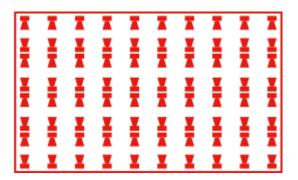
Either fit eighty A100 (100dB(A) at 1m) units or fit just two A121 (121dB(A) at 1m) units
